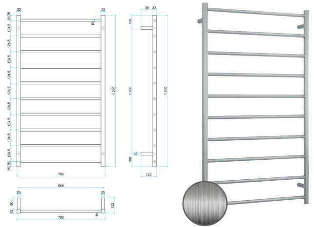
This rail has Multiflex wiring which means that there is a connection point on both the left and right hand side of the rail and the lead can be connected to either side. Being a dry electric element rail, this can be mounted either way up meaning the wiring can be from any of the four mounting points.
