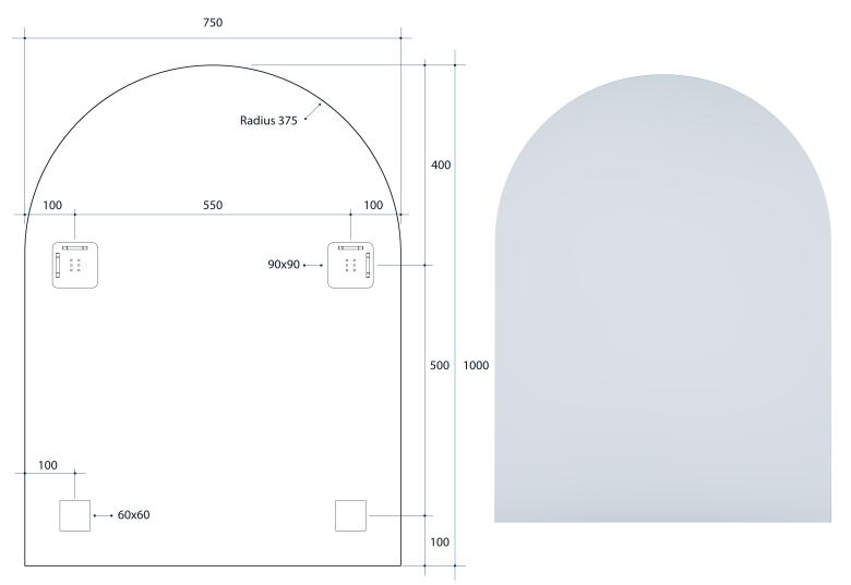
Note: All dimensions are in millimetres (mm)
