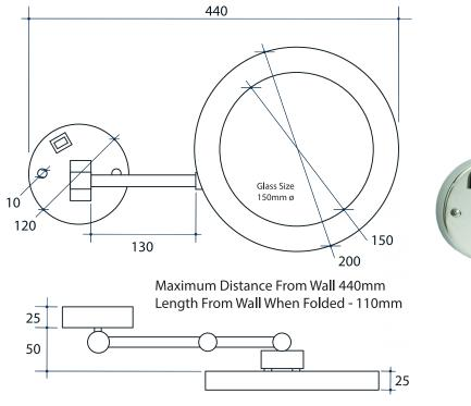
Note: All dimensions are in millimetres (mm)
