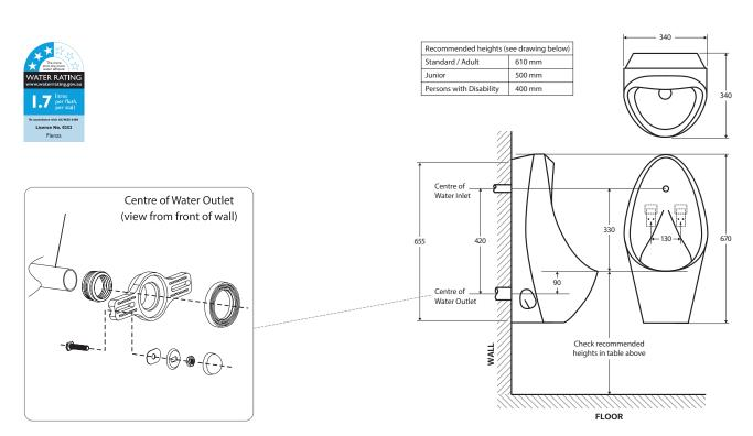
All installations should be carried out by a qualified tradesman in compliance with the National Plumbing & Drainage Code and any State or Local Authority Regulations, in accordance with AS/NZS 3500 series of standards and AS/NZA 6400. All measurements are in millimetres and are subject to change without notice. For ceramic products, please allow +/- 10 mm tolerance for manufacturing variance. Please refer to fienza.com.au for the latest product specification.
